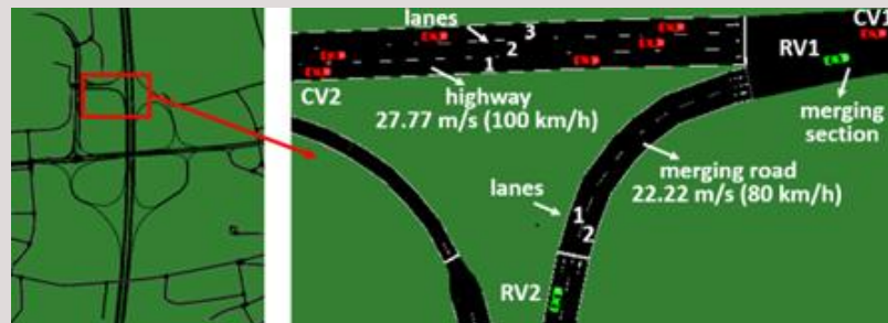
Fig. 2: Road network and traffic demand for a highway merging scenario in SUMO for merging and lane change cooperative maneuvers.
